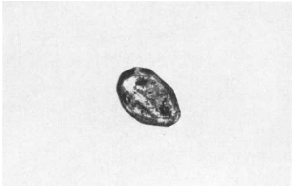
FIG. 44 Almandine garnet from Madagascar. An inclusion of a slightly rounded zircon crystal. 110 ×
