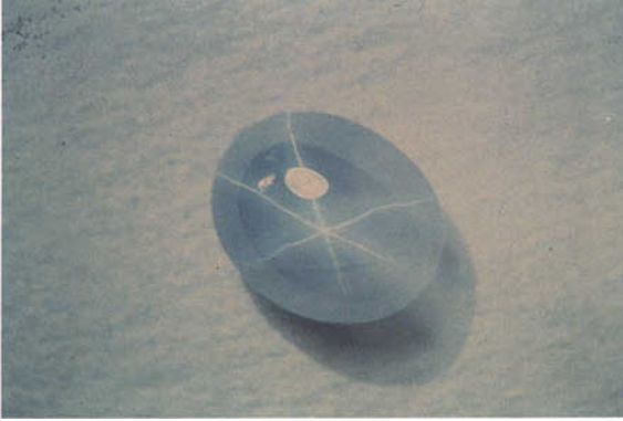
FIG. 12. Asterism added by a surface diffusion step (process 7, Table 1).
