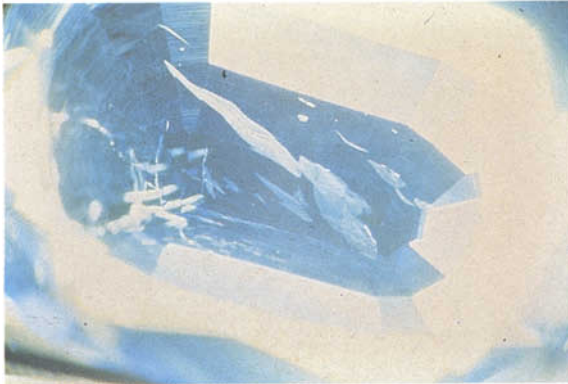
FIG. 15. Induced fingerprint inclusion in heated Verneuil synthetic sapphire.
