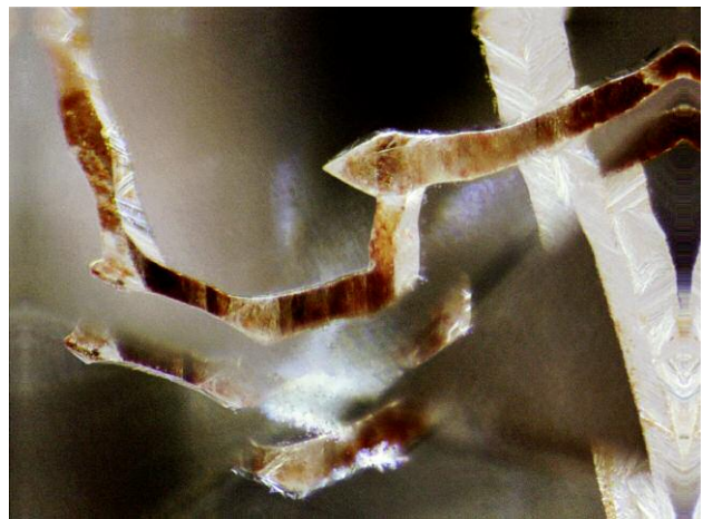
Figure 4. Rare etch channel with a pyramidal termination in a 1.77 ct type IIa diamond. Note the lateral continuation of the dissolution. Photomicrograph by Aurélien Delaunay; field of view 1.39 mm.
