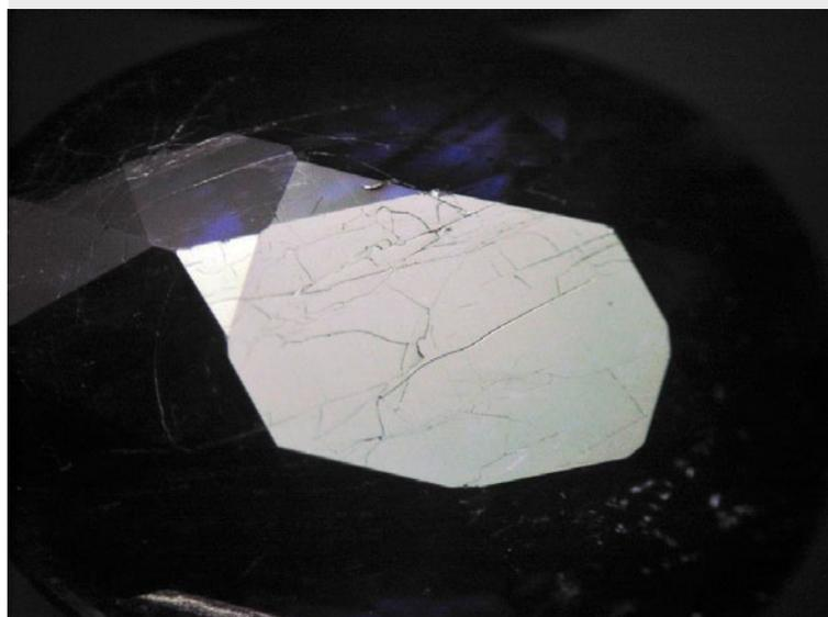
Figure 18. Table facet of one cobalt-doped glass-filled sapphire before (top) and after (below) heating with a jeweler's torch. Photos by Thanong Leelawatanasuk.
