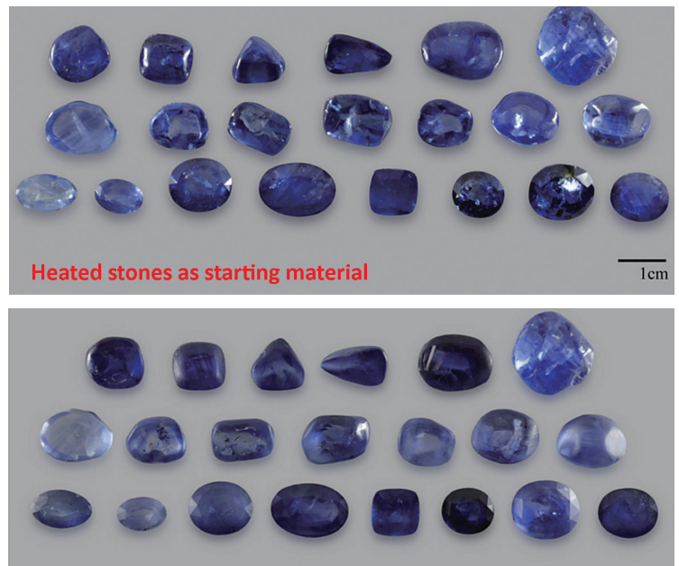
Figure 3: Top: before; Bottom: after treatment: variability of resulting colors, with some stones with no color change or even lighter color after the treatment. (Image from Choi et al. 2018. (Photos: P. Ounorn)
